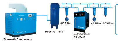
Pressure dew point: 2~10°C Oil content: 0.003ppm Dust content: <0.01µm For diving operation, breathable air,food compound, dentistry, cosmetics,hyperbaric oxygen chamber
