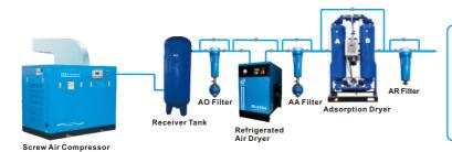
Pressure dew point: -20~-70°C Oil content: 0.001ppm Dust content: <0.01µm For print, film industry, nuclear industry, aerospace industry, precision control instrument
